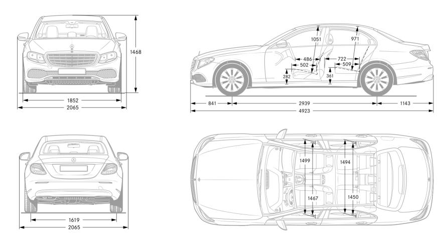
All figures in millimetres. The illustrated dimensions are average values. They are valid for vehicles in basic specification and in unladen condition.
